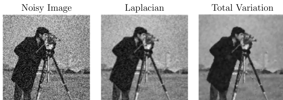
Figure 7.18: Comparison denoising an image with Laplacian and total variation regularization (images from Mathworks Matlab manual).
