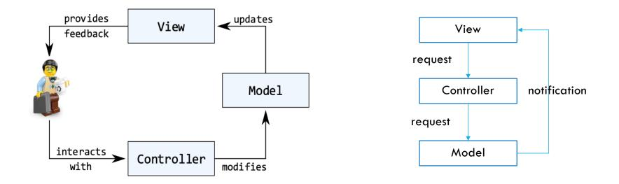
MVC is sort-of a layered architecture. Requests go down, notifications come back up.
