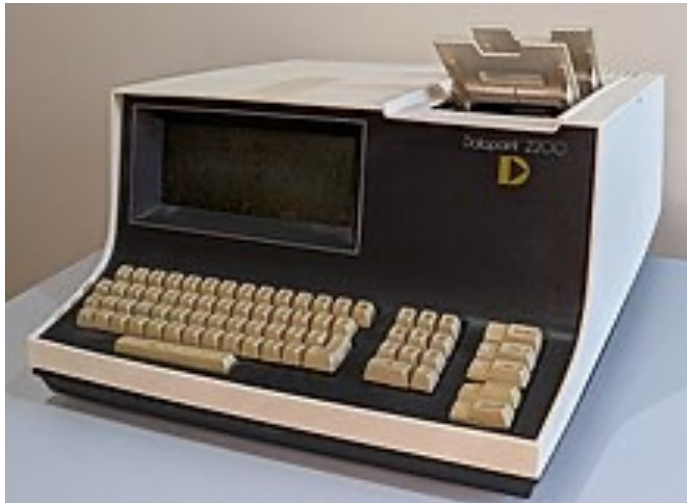
The CTC Datapoint 2200 would load simple programs into e.g., terminal protocols, but was essentially a fancy terminal.
