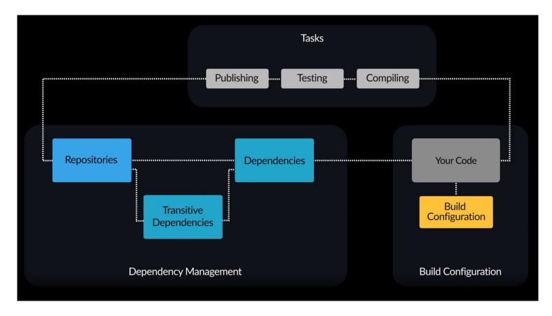
The pillars of a build system: managing code and dependencies, tasks that define actions to take, and configuration scripts that determine how to run these tasks.
