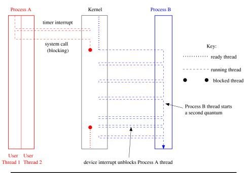
Once Process A's thread blocks, only Process B's thread can run.
