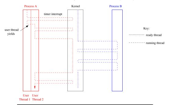
Process A has two user-level threads, but only one kernel thread.
