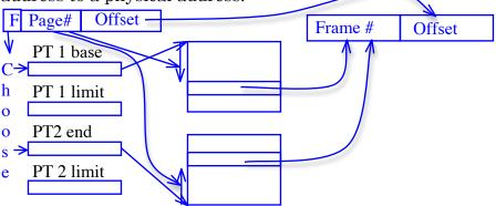
pick PT1 or PT2 based on flag; check page number against limit register, index into page table (forward for PT1, backward for PT2), check valid bit in entry, concatenate frame number from entry with offset from address.
