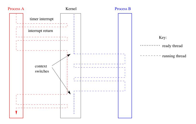
Two process' threads timesharing a single CPU.
