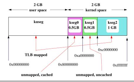
In OS/161, user programs live in kuseg, kernel code and data structures live in kseg0, devices are accessed through kseg1, and kseg2 is not used.
