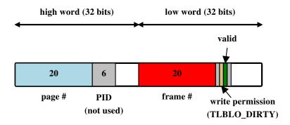
The MIPS TLB has room for 64 entries. Each entry is 64 bits (8 bytes) long, as shown. See kern/arch/mips/include/tlb.h
