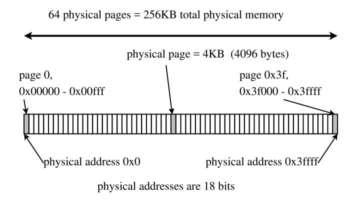
Physical memory is divided into fixed-size chunks called *frames* or *physical pages*. In this example, the frame size is  $2^{12}$  bytes (4KB).
