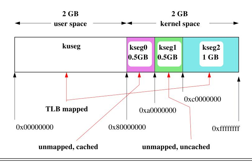
In OS/161, user programs live in kuseg, kernel code and data structures live in kseg0, devices are accessed through kseg1, and kseg2 is not used.
