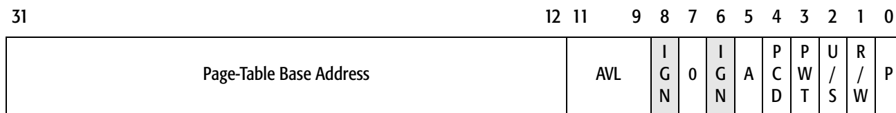
Figure 5-5. 4-Kbyte PDE—Non-PAE Paging Legacy-Mode
