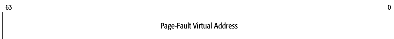
Figure 8-1. Control Register 2 (CR2)
