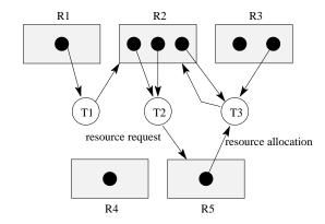
The deadlock detection algorithm will terminate with  $f_1==f_2==f_3==$  false, so this system is deadlocked.
