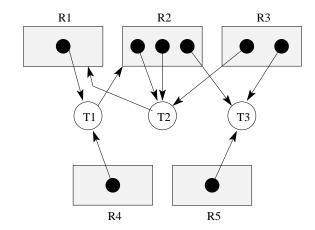
This system is not in deadlock. It is possible that the threads will run to completion in the order  $T_3$ ,  $T_1$ ,  $T_2$ .
