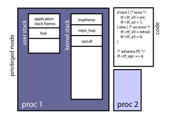
sys\_fork returns to syscall. syscall sets up the return value/error code and result. It also increments the PC.
