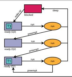
T3 is woken by T1 causing T1 to be preempted. Many variants of MLFQ will preempt low-priority threads when a thread wakes to ensure a fast response to an event.
