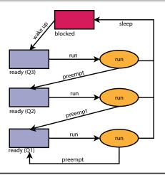
When do threads in Q1 run if Q3 is never empty? To prevent starvation, all threads are periodically placed in the highest-priority queue.
