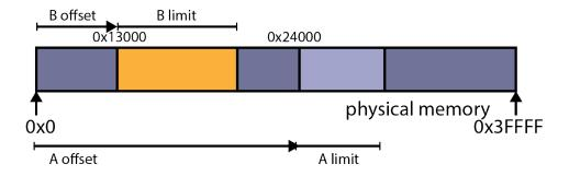
offset, or, relocation (R) is the position in physical memory where the processes memory begins. **limit (L)** is the amount of memory used by the process. The MMU has a register for each. Given virtual address v:
