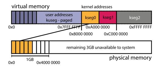
Addresses within kseg0 are for the kernel's data structures, stacks, and code. To translate kseg0 addresses to physical ones  $\frac{\text{subtract}}{\text{0x}8000\ 0000}$  from the virtual address.
