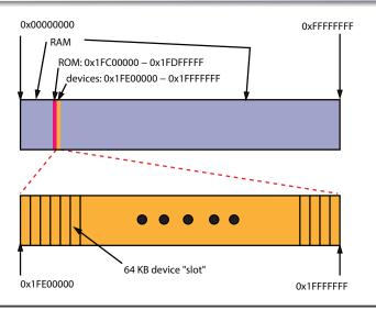
Each device is assigned to one of 32 64KB device "slots". A device's registers and data buffers are memory-mapped into its assigned slot.
