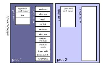
Thread context is restored from trapframe. Switch from kernel to user stacks. Switch to unprivileged mode. User code continues execution.
