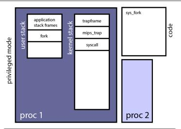
syscall, the system call dispatcher, calls the appropriate handler for the system call code provided in v0. In this case, sys\_fork is called.
