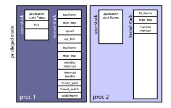
The interrupt handler returns to mainbus\_interrupt.
