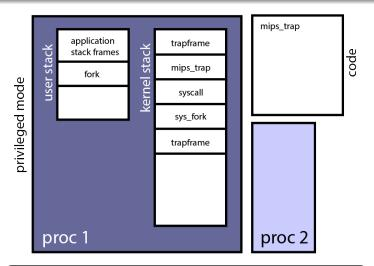
mips\_trap determines which exception has been raised. In this case, a timer interrupt.
