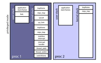
mainbus\_interrupt returns to mips\_trap.
