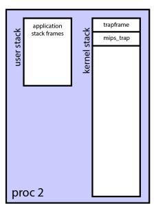
${\tt mainbus\_interrupt\ returns\ to\ mips\_trap}.$
