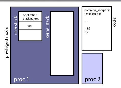
mips\_trap returns to common\_exception. The trapframe data is restored. Switch from kernel to user stack. Switch to unprivileged mode (rfe). User code continues execution.
