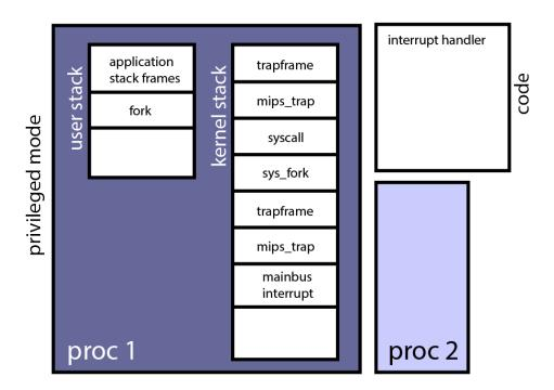
The device interrupt handler runs. Thread quantum has expired.
