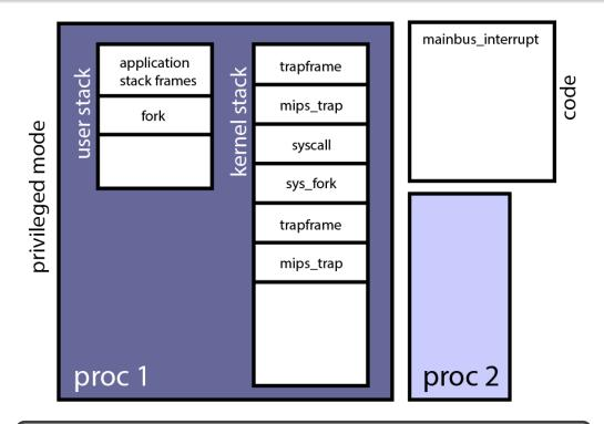
mainbus\_interrupt determines which device threw the interrupt, then calls the appropriate handler.
