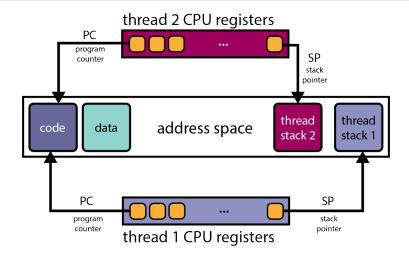
Conceptually, each thread executes sequentially using its private register contents and stack.
