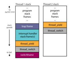
Thread 2 is now **RUNNING**, Thread 1 is now **READY**. Thread 2 returns from low-level context switch, restoring callee-save registers.
