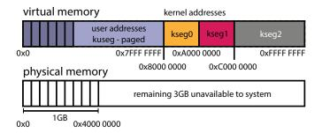
$\mbox{Sys}/161$  only supports 1GB of physical memory. The remaining 3GB are not available/usable. The kernel's virtual memory is divided into three segments:
