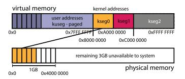
Addresses within kseg0 are for the kernel's data structures, stacks, and code. To translate kseg0 addresses to physical ones **subtract** 0x8000 0000 from the virtual address. **kseg0 maps to the first 512MB** of physical memory, though it may not use all of this space.
