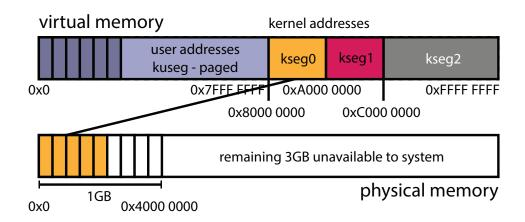
Addresses within kseg0 are for the kernel's data structures, stacks, and code. To translate kseg0 addresses to physical ones **subtract** 0x8000 0000 from the virtual address.
