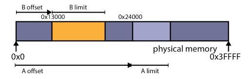
offset, or, relocation (R) is the position in physical memory where the processes memory begins. limit (L) is the amount of memory used by the process. The MMU has a register for each.
