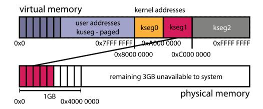
Addresses within kseg1 are for accessing devices. To translate kseg1 addresses to physical ones **subtract 0xA000 0000** from the virtual address.
