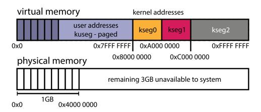
$\mathrm{Sys}/161$  only supports 1GB of physical memory. The remaining 3GB are not available/usable. The kernel's virtual memory is divided into three segments:
