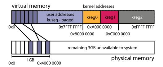
User virtual memory, kuseg, is paged. The kernel maintains the page-to-frame mappings for each process. The TLB is used to translate kuseg virtual addresses to physical ones.
