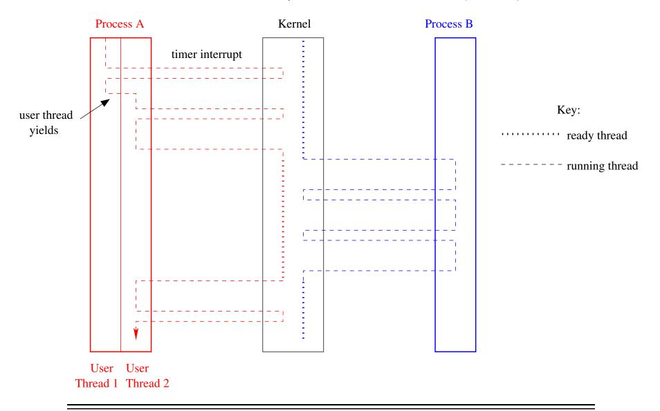
Process A has two user-level threads, but only one kernel thread.
