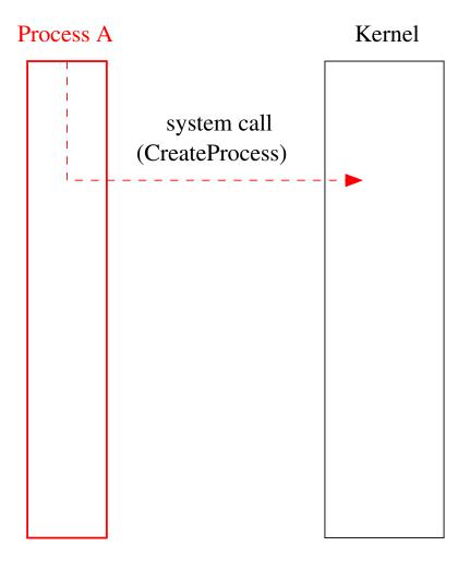
Parent process (Process A) requests creation of a new process.
