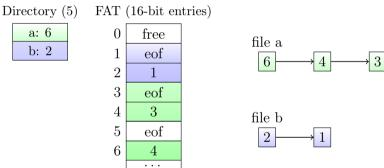
Still do pointer chasing, but can cache entire FAT so can be cheap compared to disk access
