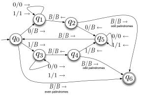
Seems complicated, but not that bad. The top branch matches 0s at both ends of the word, while the bottom branch matches 1s.
