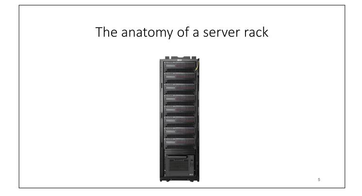
We put multiple servers in a server rack. There is a network switch that connects the servers in a rack. This switch also connects the rack to other racks.
