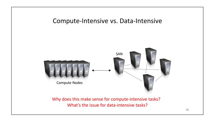
This makes sense for compute-intensive tasks as the computations (for some chunk of data) are likely to take a long while even on such sophisticated hardware, so the communication costs are greatly outweighed by the computation costs. For data-intensive tasks, the computations (for some chunk of data) aren't likely to take nearly as long, so the computation costs are greatly outweighed by the communication costs. Likely to experience latency and bottleneck even with high speed transfer.
