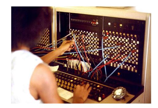
Calls are connected with cord pairs at a telephone switchboard.
