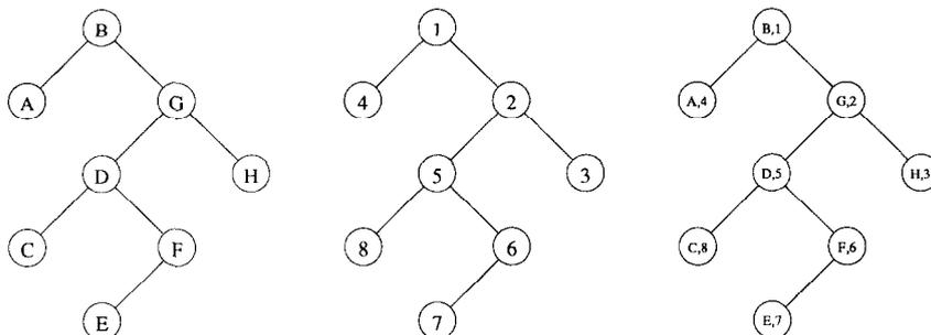
Fig. 2. Binary search tree, heap and treap.
