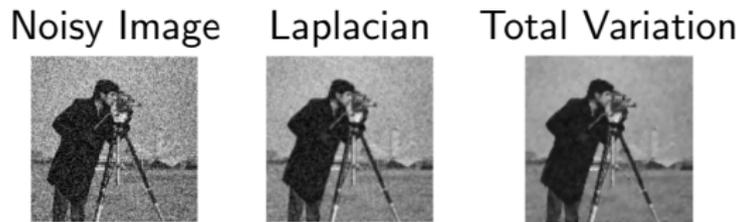
**Figure:** Comparison denoising an image with Laplacian and total variation regularization (images from Mathworks Matlab manual).
