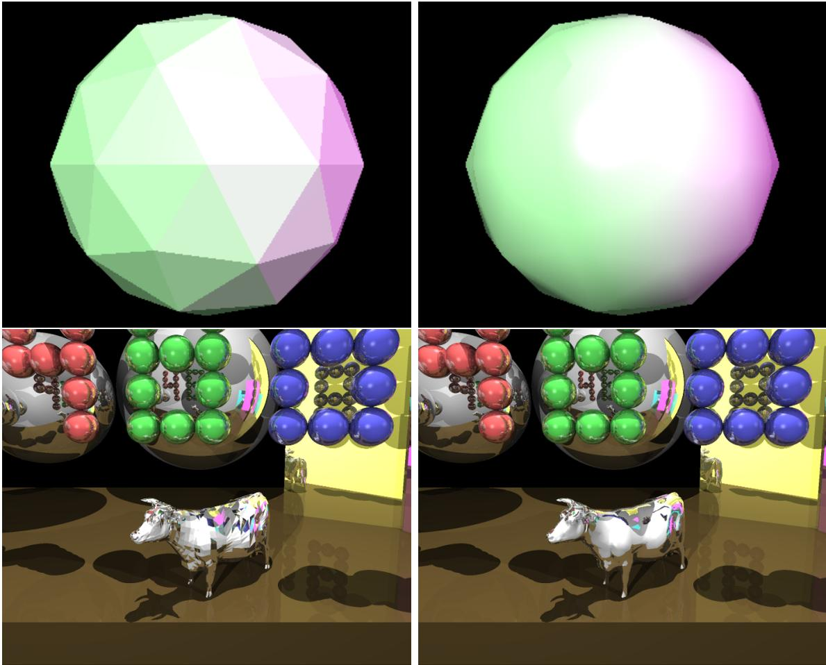
Figure 4: Comparison between renders using face-wise triangle normals (left two) and with Phong shading (right two).
