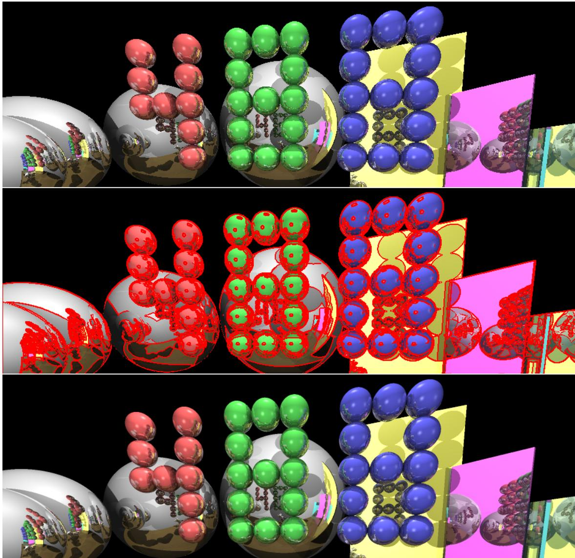
Figure 1: Edge detection using a threshold value on any of the colours, showing no antialiasing (top), edge detection (middle), and 2x AAA (bottom).
