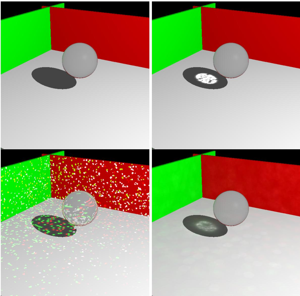
Figure 10: Each step of the photon-mapping process: before (top-left), caustics photons (top-right), global illumination photons (bottom-left), sampled and finished (bottom-right).
