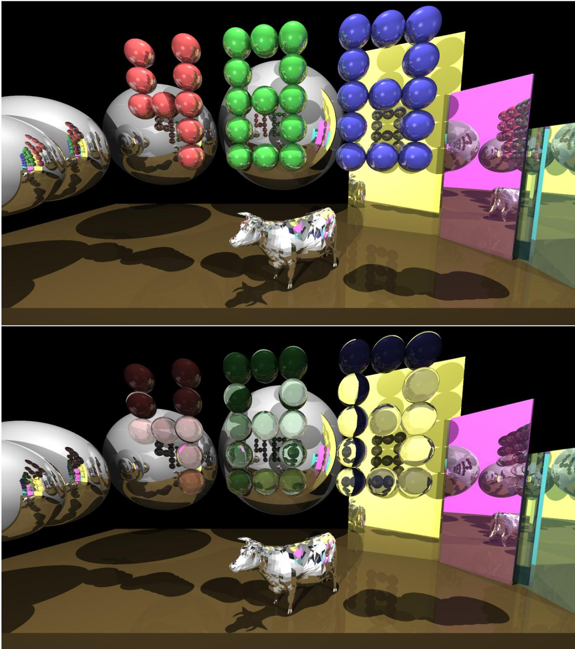
Figure 3: Comparison between renders with no refractions (top) and multiplicative refractions turned on for the spheres comprising the “488”, using refractivity 0.9 and refractive index 1.2 (bottom).
