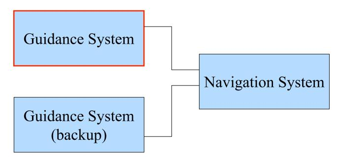
(2) The guidance system shuts down. Control passes to the backup guidance system.
