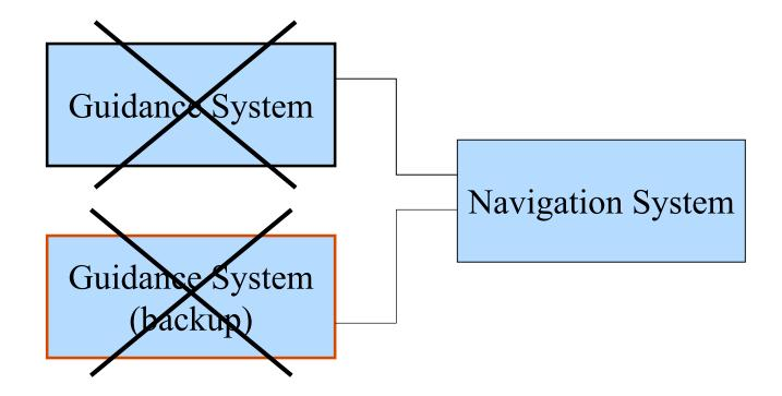
(4) The backup guidance system warns the navigation system that a run-time error has occurred.
