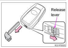
After using the mechanical key, store it in the electronic key. Carry the mechanical key together with the electronic key. If the electronic key battery is depleted or the entry function does not operate properly, you will need the mechanical key.  $(\rightarrow P. 726)$
