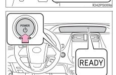
Depress Brake Pedal and Push Power Switch to Start
